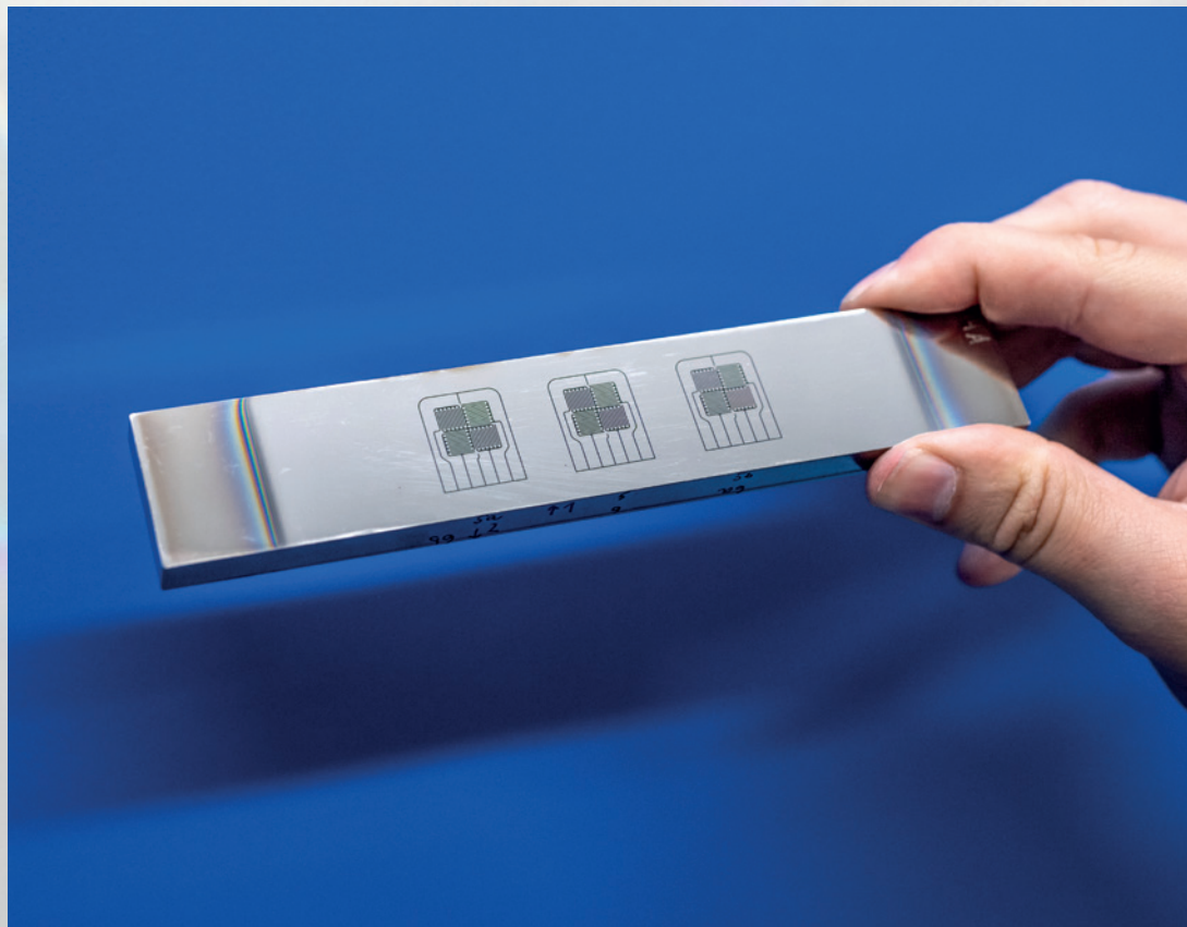
The photo shows a prototype of a strain sensor, used in fields like robotics. It is the result of extremely precise micromachining, where the laser had to evaporate a layer just 250 nanometers thick without damaging the underlying ceramic layer.
