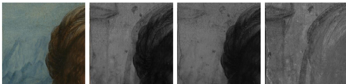
Figure. Pentimenti visualiation using deep neural networks. Our experiment with the 16th century wooden desk painting attributed to Leonardo da Vinci. Left: RGB image, middle-left: a reflectogram centered at wavelength \lambda=1050\text{nm} , middle-right: output of ANN extrapolation, right: difference between the measured and the extrapolated outputs; the information gain.
